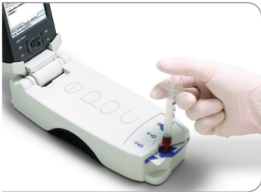
Immediate introduction of a patient's blood sample into a test card minimizes pre-analytical sample handling errors. All that's required is a 100 µl blood sample.
